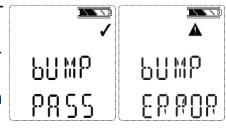
NOTE: If the device fails the Bump Test, take it out of service and notify BFD MGD Technician!
